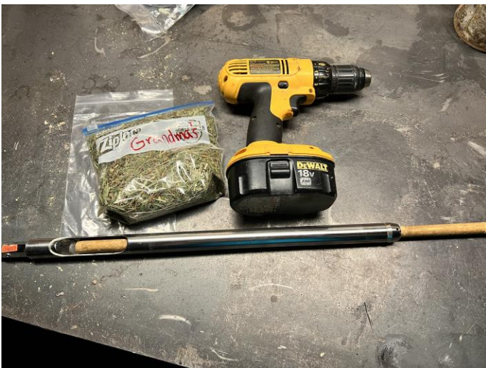
Picture 1 (drill, corer, quart-sized bag for sample)
