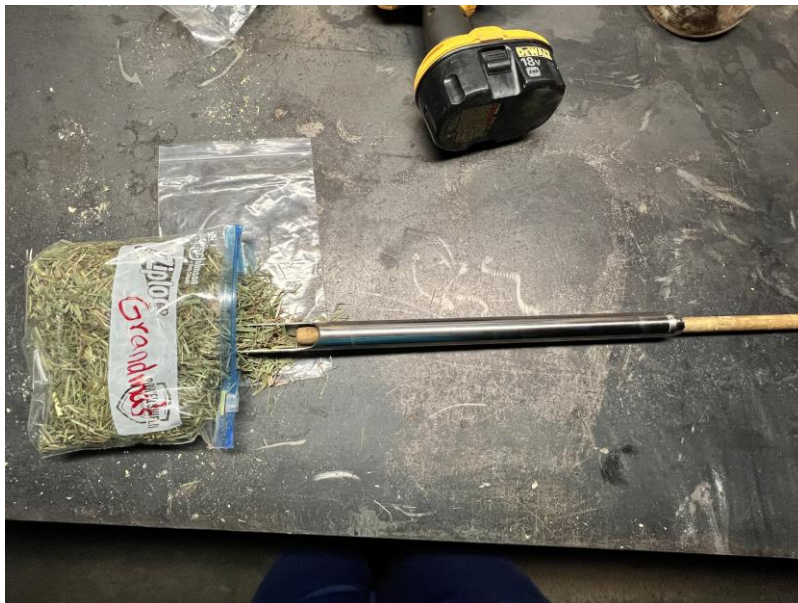
Picture 5 (plunge hay sample into plastic bag through small hole)
