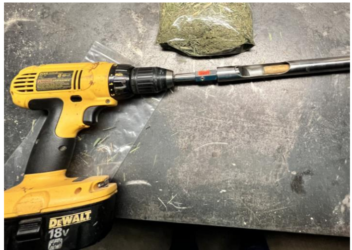
Picture 2 (corer connected to drill)
